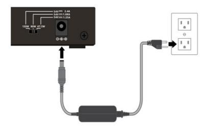
1. Power down the switch and disconnect the power cord.
