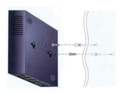
Note: You can mount the switch with the Ethernet ports facing down (at the bottom) as shown, or with the Ethernet ports facing up.
