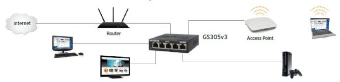
In the Sample connections diagram, the entire network is deployed indoors. If you want to connect an outdoor device to the switch, cable the switch to an Ethernet surge protector that supports the same speeds as your switch, and then cable the surge protector to the outdoor device.
