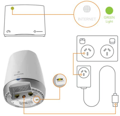
Wait ten minutes for the CloudMesh Satellite to initialize and then check the light status. A solid white or blue light means the satellite has been paired with the Gateway and is ready to use.
