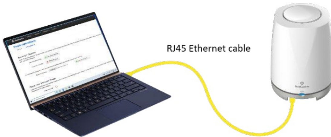
Figure 7 – RJ45 Ethernet cable connecting PC with NC-01
