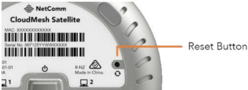
Figure 14 – Location of reset button on bottom
