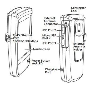
The AirCheck G2 is a comprehensive, hand-held tool for network professionals to test and troubleshoot the latest wireless networks. The AirCheck G2 operates on 802.11b/g/n networks in the 2.4-GHz band and 802.11a/n/ac networks in the 5-GHz band. It offers the following test types:
