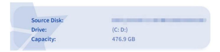
Target disk: New disk used for data migration. The disk capacity must be larger than that of the source disk; otherwise, the migration fails.
