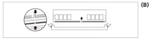
3. Match the notch on the edge of a golden finger with sthe lot, press both ends of the DRAM module ,and push it into the motherboard slot until you hear a "PA" sound. (C
