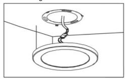
Step 5: Rotate the LED downlight on the mounting bracket to secure position.
