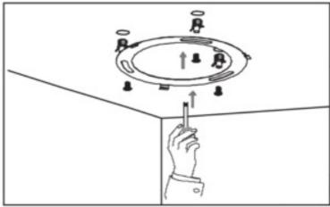
Step 2: Feed the mains AC wires into the driver connector block, connect the surface circular and driver
