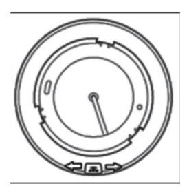
Step 4: Fit LED surface circular onto the mounting bracket
