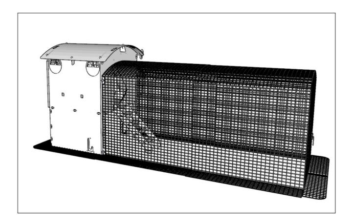
This product has been Hot dipped galvanized in a bath of molten zinc, which provides a corrosion-resistant layer that is effective in most climates. This is to protect the metal from rust if paint is chipped off.
