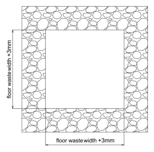
• Install floor waste as above picture. Note: it can be installed 2 ways: tile insert placement and normal placement.
