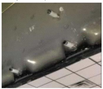
• **Step 5:** An additional person is recommended for this step. Carefully install the step assembly to the three factory attachment points using the provided M8 flanged hex nuts. Leave your finger tight for now.
