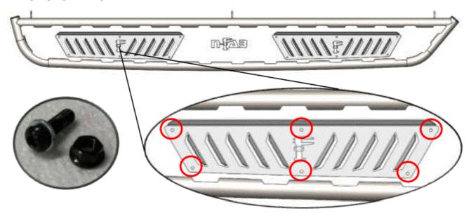
• Step 3: Install the supplied rocker panel brackets (x6) to the attachment points located on the backside of the main tube (Driver/Passg) using the supplied 3/8"x 1" carriage bolts and 3/8" flanged nuts. Leave your finger tight for now. \*\*\* NOTE: The mounting bracket will mount forward on the tube attachment with the threaded part of the bolt facing toward rear of the vehicle
