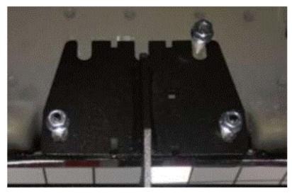
• Step 6: There will be ½" of adjustment in the (x3) mounting bracket. Adjust to desired position and tighten to (20 ft,/lbs). Then tighten body mount brackets to (17-20 ft./lbs)
