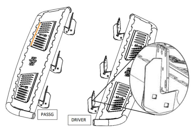
• Step 4: On the inside Rocke panel there will be three attachment points consisting of three 8m m studs coming out from the panel. These studs may be covered in paint and will need to be cleaned before the installation.
