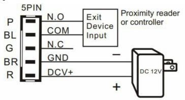
• B. Fail secure type electric lock.
