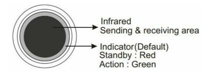
In order to ensure the operation of the infrared switch, please make sure no objects or any obstacles are within 30cm & 60° on the left and right of the front panel of the switch to avoid any interference.
