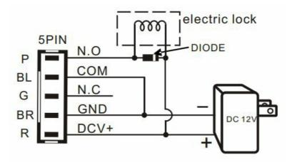
• **D.** Connect Relay (Power > DC30V >or Current 1A)
