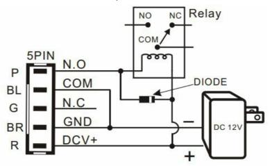
Please connect a diode when the control terminal is loading in order to absorb any surge to prevent damage to the sensor.
