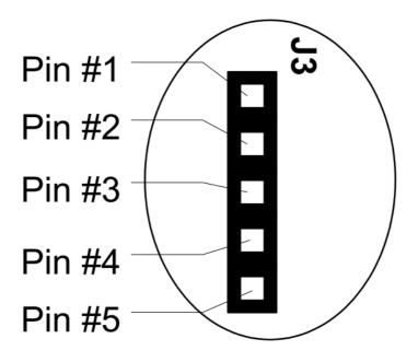
When not used for programming, jumper is placed between pin 4 & 5
