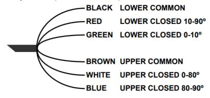
Auxiliary switch rating: 5 Amp resistive, 250 Vac
