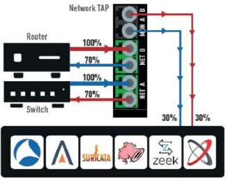
Network Packet Broker / Monitoring Device / IDS / IPS
