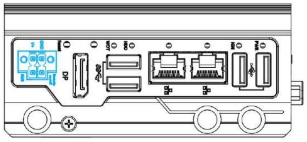
The system accepts DC power input from 12 to 20V via a 4-pin terminal block. The terminal block can also accept ignition signal input (IGN).
