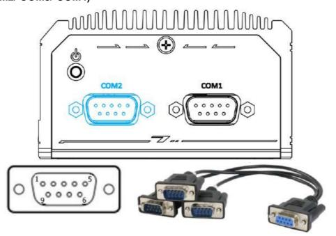
COM2 is a 3-port 9-wire RS-232 port. You can directly connect to one external device, or use an optional 1-to-3 Y-cable to connect up to three devices. The following table describes the pin definition of the DB9 connector as well as the Y-cable.
