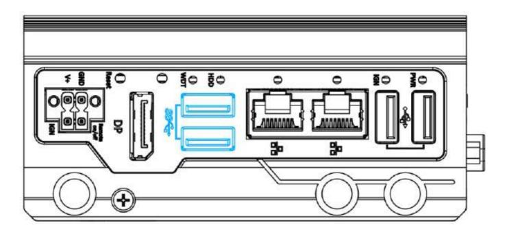
The system offers two USB 3.0 (SuperSpeed USB) ports on its front panel. They are implemented by a native xHCI (eXtensible Host Controller Interface) controller and are backward compatible with USB 2.0, USB 1.1 and USB 1.0 devices. Legacy USB support is also provided so you can use a USB keyboard/mouse in a DOS environment.
