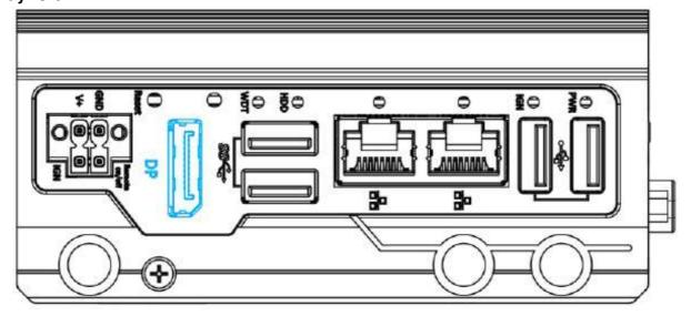
The system has a DisplayPort (DP) output which are digital display interfaces that mainly connect video source and carry audio to a display device. When connecting a DP, it can deliver up to 4K UHD (4096 x 2160 @ 30Hz) in resolution. The system is designed to support passive DP adapter/ cable. You can connect to other display devices using DP-to-HDMI cable or DP-to-DVI cable.
