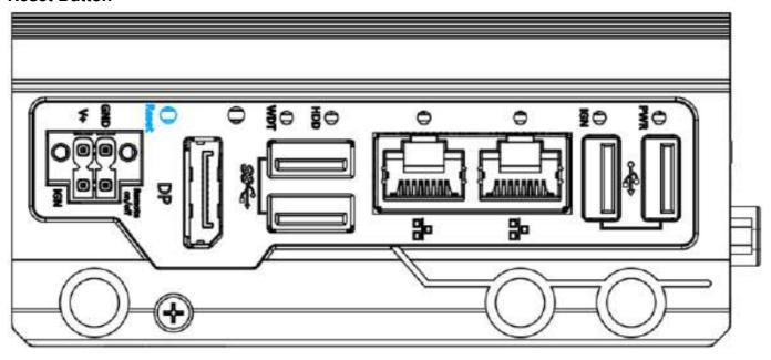
Use to manually reset during system halt or malfunction. To reset, please use a pin-like object (eg. tip of a pen) to access the reset button.
