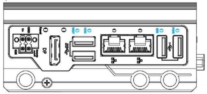
There are four LED indicators on the front panel: PWR, HDD, WDT and IGN. The descriptions of these four LEDs are listed in the following table.
