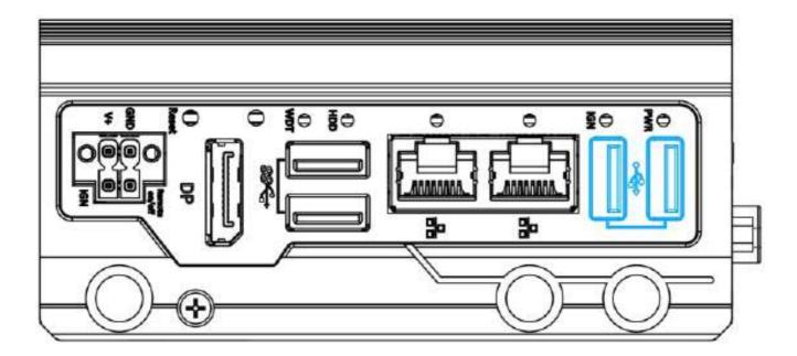
The USB2.0 ports are implemented via native xHCI (eXtensible Host Controller Interface) and are backward compatible with USB 1.1 and USB 1.0 devices. Legacy USB support is also provided so you can use a USB keyboard/ mouse in a DOS environment. xHCI driver is supported natively in Windows 10, therefore you do not need to install xHCI driver to utilize USB functions.
