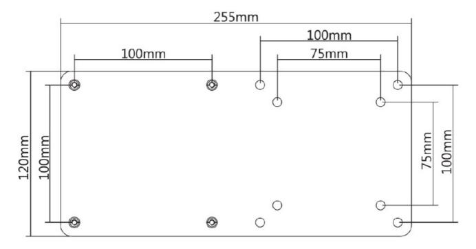
The Neomounts by Newstar THINCLIENT-01 allows you to mount a thin client PC to a monitor/TV mount with VESA75/100 holes. A thin client mount creates a need and tidy workplace because the PC is stored behind the screen and doesn't use any valuable desk space. Keep the workplace clean without computers on the desk.
