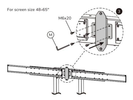
**STEP 3**Install the adapter brackets and use spacers if necessary.
