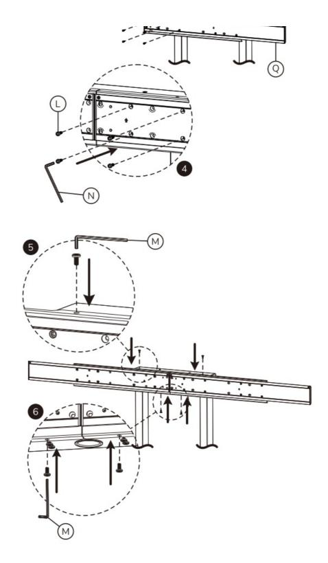
Assemble the adapter plate according to the indicated position on the plates
