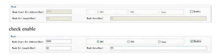
Only check enable can do mask operation For example, EPC mask Choose EPC area
