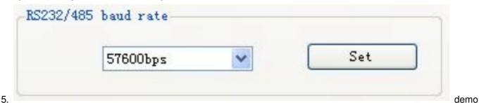
software start run, default use the baud rate 57600 to open COM port, reader power on, reader baud rate default is 57600. After change the baud rate, reader use the new baud rate until power off. Close port and open port, the baud rate no change. The demo software will use the new baud rate, until close the demo software.
