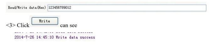
Note: write data can be used to change the EPC number
