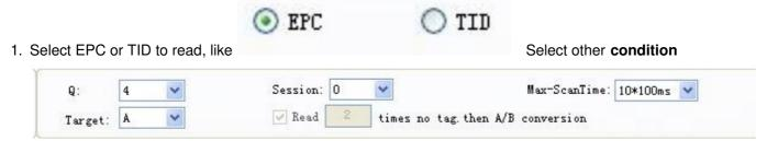
**Note:** about Q, S choice, a single tag or less number must be S0, a lot of tag queries using S1 or S2, S3. 2Q equal tag number is better. If it is a single query effect must use S0
