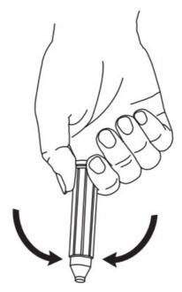
6. With the instrument held upright, press the eject button and insert the sampler.
