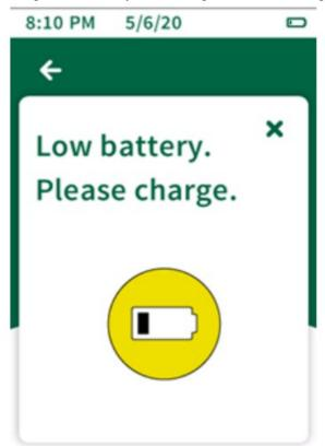
Error 07: The unit battery is depleted, the unit is shutting down. Connect the unit to the USB charger.
