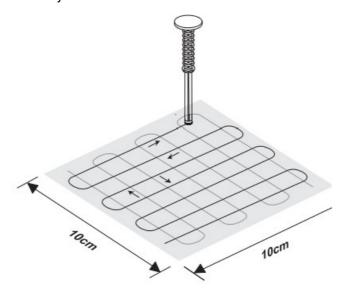
4. Hold the sampler vertically and insert into unibody, and fully depress to activate. Note: The sampler must be held vertically.
