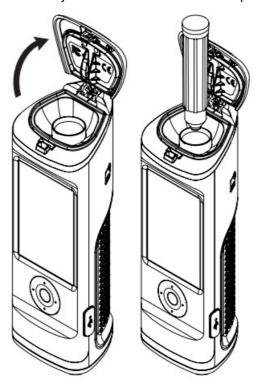
7. Close the door to depress the sampler and begin test. Note: keep instrument upright while the sample is being read.
