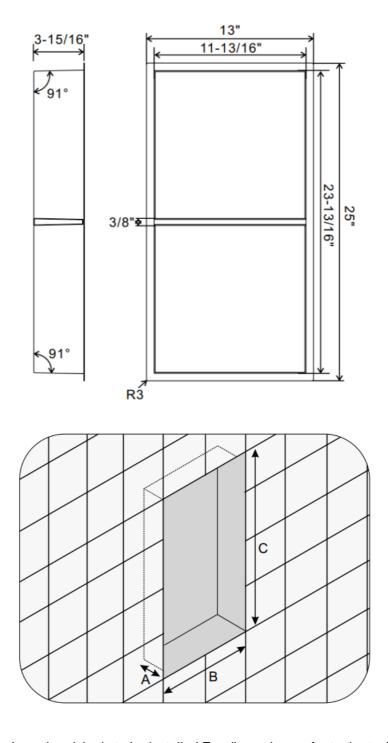
1. Dig a hole in the wall where the niche is to be installed. For dimensions, refer to the technical drawing shown
