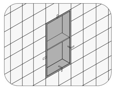
4. Use adhesive tape to adhere the niche to the wall and tear off the tape after the glue has been fixed for 24 hours.
