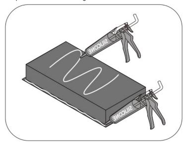
2. Seal the edges of the back of the mounting niche.
