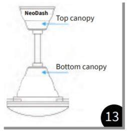
13. Position top and bottom canopy. Keep gap of min 5 mm between bottom canopy and motor
