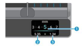
Divider allows the user to divide a certain distance (slider's distance) into 2-12 sections.
