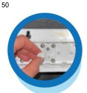
4 Place the plug in the outlet where the red drain line was removed from
