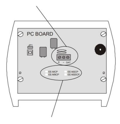
The keypads referred to are distinguishable by the markings 'EE-MCP, EE-M2CP, EE-M9CP and EE-M20CP on the PC board, below the terminal connector.
