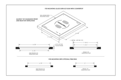
Drawing for the control panel cut-out.
