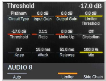
At the top of the display, the current parameter line shows the last controlled parameter. In this case the compressors Threshold parameter.
