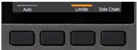
The 4 LED buttons below the 12 pots can also be used for parameter control. If a button is illuminated, it's controlling a parameter.
