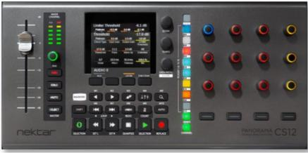
The display shows the parameter assigned to each of the 12 rotary controls.
