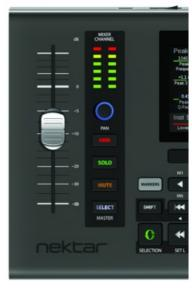
**Fine Control**: The fader can control parameters at 14 bit resolution. Hold the Fine (magnifier) button while moving the fader. To reposition the fader without affecting the parameter, hold [Fine]+[Mute] and move the fader.
