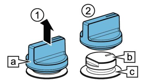
To put the control knob back on, press it on at its original position.
