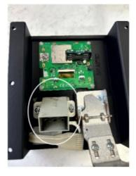
5. The new front panel is ready to place it to vending machine with 6 screws.
