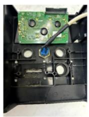
3. Place back all plastic push buttons and springs to new front panel.
