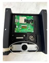
4. Screw back money back button hinge mechanic and coin slide tube.
