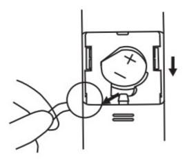
To replace the batteries, slide off the battery compartment backplate to open the battery compartment, insert new batteries (matching the polarity (+/-) as indicated), and close the battery compartment.
