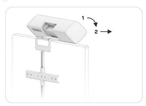
• Warning: Do not leave Neat Bar in a max tilted position with the red indicator showing as it is not secured by the lock spring.
