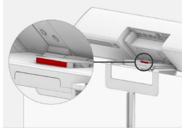
**Warning:** Do not leave Neat Bar in a max tilted position with the red indicator showing as it is not secured by the lock spring.
