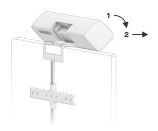
To release Neat Bar from the selected mounting option, tilt the unit to maximum tilt (1) and carefully slide the unit towards you (2).
