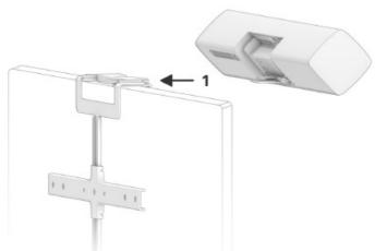
Slide Neat Bar onto the selected mounting option (1). When fully inserted tilt Neat Bar back to horizontal and check if it is secure by carefully pulling it towards you.
