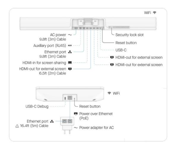
The 16.41t (5m) Ethernet Cable provided is not to be used for InovSI installation. In-wall cable routing &noted oily be performed by qualified personnel using appropriate equipment.
