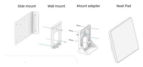
Hook the mount adapter onto the wall mount and secure with the hex wrench.
