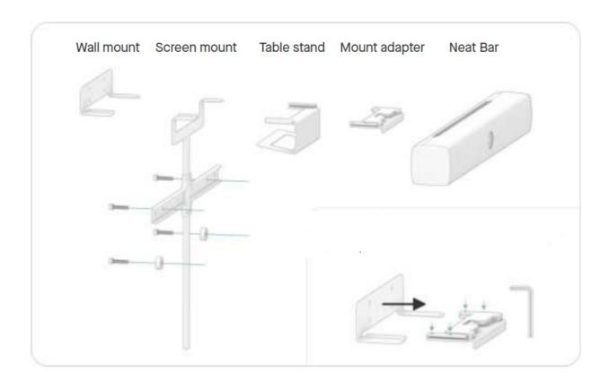
Slide the selected bracket onto the mount adapter and secure with the hex wrench. Screws for mounting to the wall are not included. Mounting on a wall should only be performed by qualified personnel in line with applicable facility and state regulations. The wall and the mounting equipment must safely withstand the load of the product.
