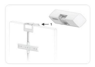
Slide Neat Bar onto the selected mounting option (1). When fully inserted tilt Neat Bar back to horizontal and check if it is secure by carefully pulling it towards you.
