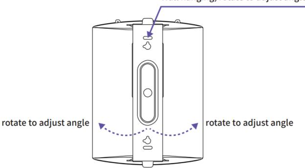
When the ASP110 is installed at the same height as the A50, in the vertical mounting mode, sometimes it is hoped that the audience will have a better voice experience, so speaker should be tilted downward for sound reinforcement. However, the angle cannot be adjusted downward in the vertical mounting mode, and other installation accessories need to be purchased.
