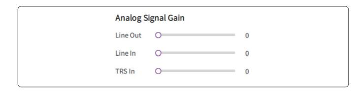
There are three analog audio interfaces on the DSP, and the analog audio gain can be set as follows: Line Out: The value is 0-14, where 10 represents 0dB, and the downward and upward changes are 5dB respectively.
