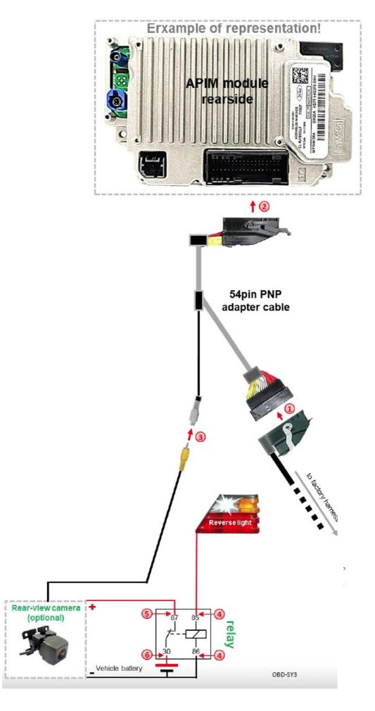
1. Disconnect the female 54-pin connector of the factory harness at the rear side of the APIM module and connect it to the male 54-pin connector of the enclosed adapter cable.
