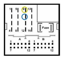
**Fabia III**Female Quadlock-connector in radio slot
