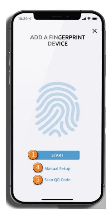
Every new keypad needs to be added in the x-manager application, before it can be used. If more than one device is connected to a single x-manager application, it is important that the first connection is established with one device at a time. The rest of the devices should not be connected to a power supply at the time of the first connection.
