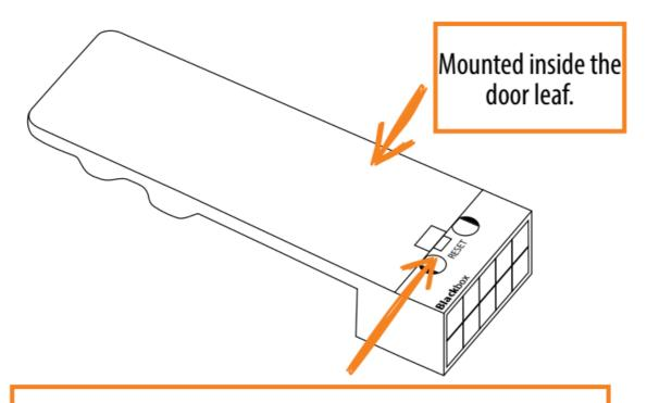
Button »R« for factory reset is located below the connector.
