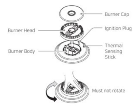
\* To prevent errors in the assembly of the burner head , place the burner head above the burner body and check if it rotates left to right.
