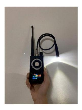
The K19 Upgrade uses a highly sensitive magnetic sensor chip, which can sense the strength of the magnetic field and accurately locate the suspicious device.
