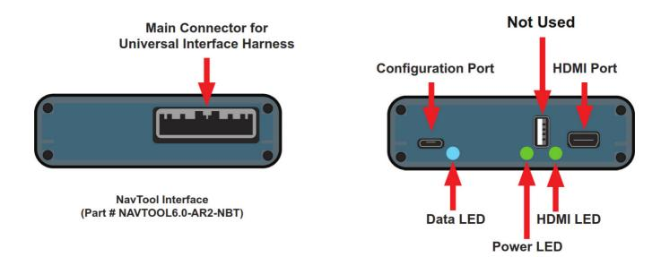
Main Connector for Universal Interface Harness- This port is dedicated for a connection of a universal wiring harness.
