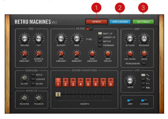
SYNTH page: Provides consistent control of parameters, whichever vintage instrument you're currently using.
