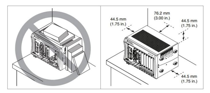
Note The previous diagram shows example dimensions, refer to your chassis user manual for specific chassis clearance dimensions.
