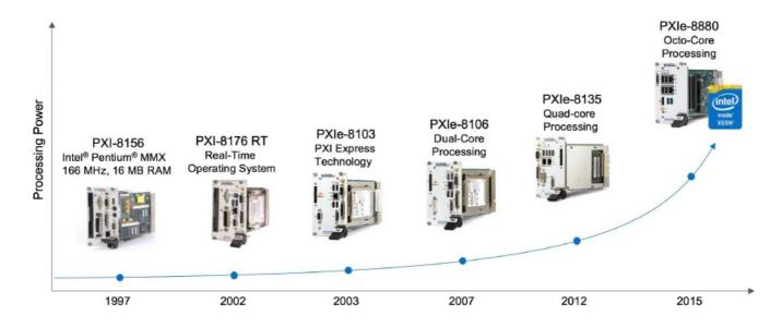
As the PCI Express standard evolved to PCI Express 3.0, PXI Express continued to take advantage of new features. The PXIe-8880 uses the advancements of PCI Express technology to offer both one x16 and one x8 Gen 3 PCI Express link for interfacing to the PXI chassis backplane.
