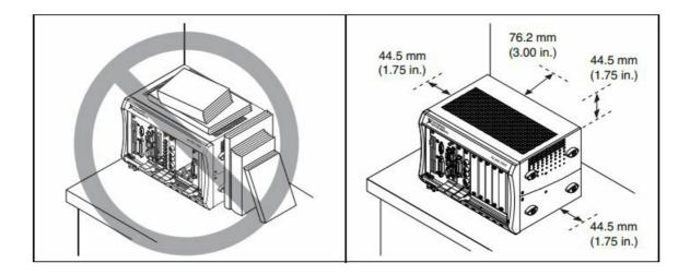
**Note:** The previous diagram shows example dimensions, refer to your chassis user manual for specific chassis clearance dimensions.
