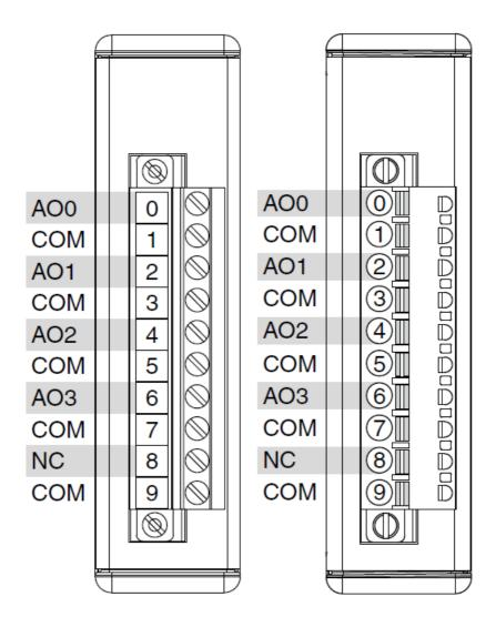
**Note:** You must use 2-wire ferrules to create a secure connection when connecting more than one wire to a single terminal on the NI 9263.
