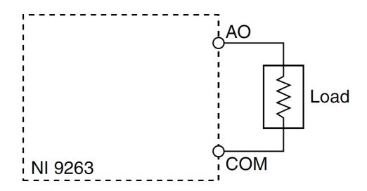
When the NI 9263 powers on, the channels output the startup voltage. You can configure the startup voltage in software.
