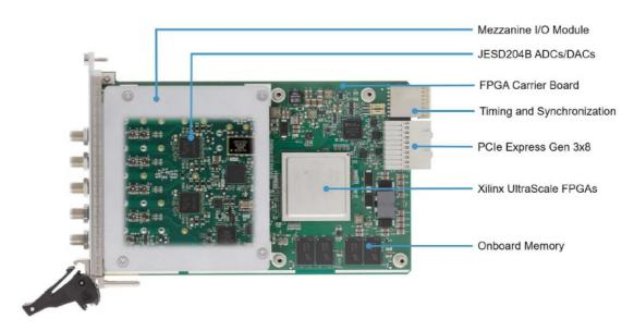
The new high-speed serial FlexRIO products are comprised of a mezzanine I/O module mated to a Xilinx UltraScale FPGA carrier.
