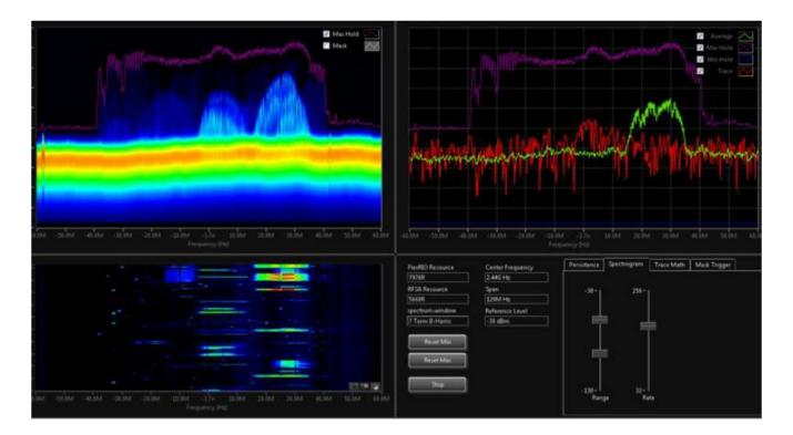
NI's Real-Time Spectrum Analyzer Reference Example processes 3.2 GB/s of data continuously on the FPGA, computing over 2 Million FFTs per second.
