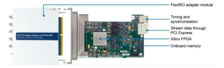
FlexRIO with modular I/O consists of a FlexRIO adapter module for analog, RF, or digital I/O, and a PXI FPGA Module for FlexRIO with LabVIEW-programmable Virtex-5 or Kintex-7 FPGAs.
