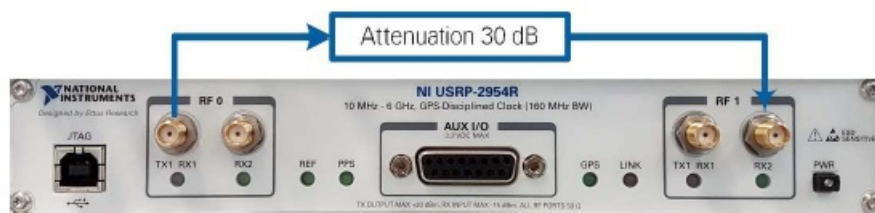
Figure 12 USRP RIO Hardware Configuration
