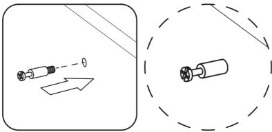
**Important Note:** Only tighten the cam bolt until it is secure. Do not over-tighten.
