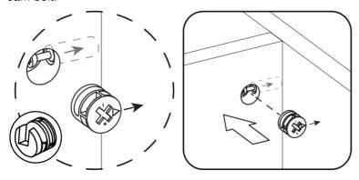
Using a screwdriver, you will turn the cam lock until it stops, usually at 90° or 180°. You will feel the panels pulling closer until they are secured.
