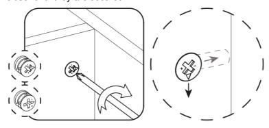
**Important Note:** Only turn the cam lock until the panels are fully engaged & feel secure. Turning too far may lead to hardware failure.
