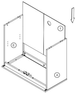
**Step 7**Attach the Bottom Panel (F) to the cabinet you assembled through Step 6, but only hand-tighten the bolts 2 rotations for this step. First insert T Nuts (11) into the side panels. Then secure the Bottom Panel (F) into place using the Long Bolts 1/4\*38mm (5) with the Spring Washers (9) and Flat Washers (8).
