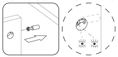
**Important Note:** When installed properly, the head of the cam bolt will be visible through the larger hole on the side of the joining panel.
