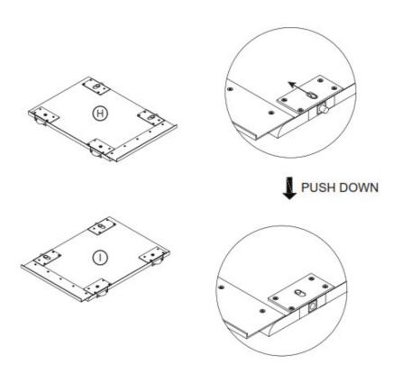
**Step 8**Line up door panel's hardware with the guide tracks on the top & bottom panels.
